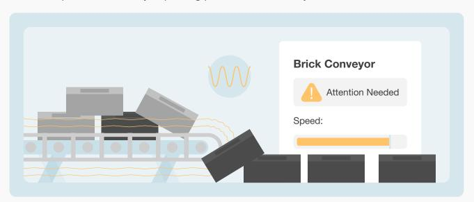
Although the machine was technically functioning as intended, the frequent micro-stoppages reduced its overall availability—the percentage of time the machine was operational during planned production. Attempts to increase machine speed worsened the issue, particularly on a newly modernized line, failing to meet production targets.
